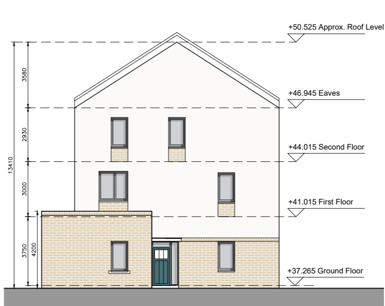
DUPLEX BLOCK M SIDE ELEVATION (NORTH)
